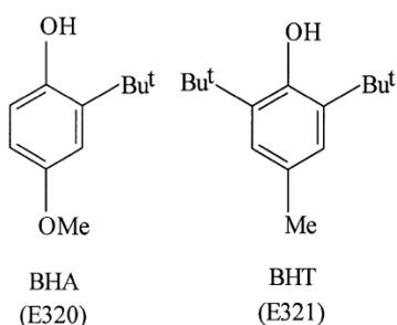
Figure 1. The structures of BHA and BHT
